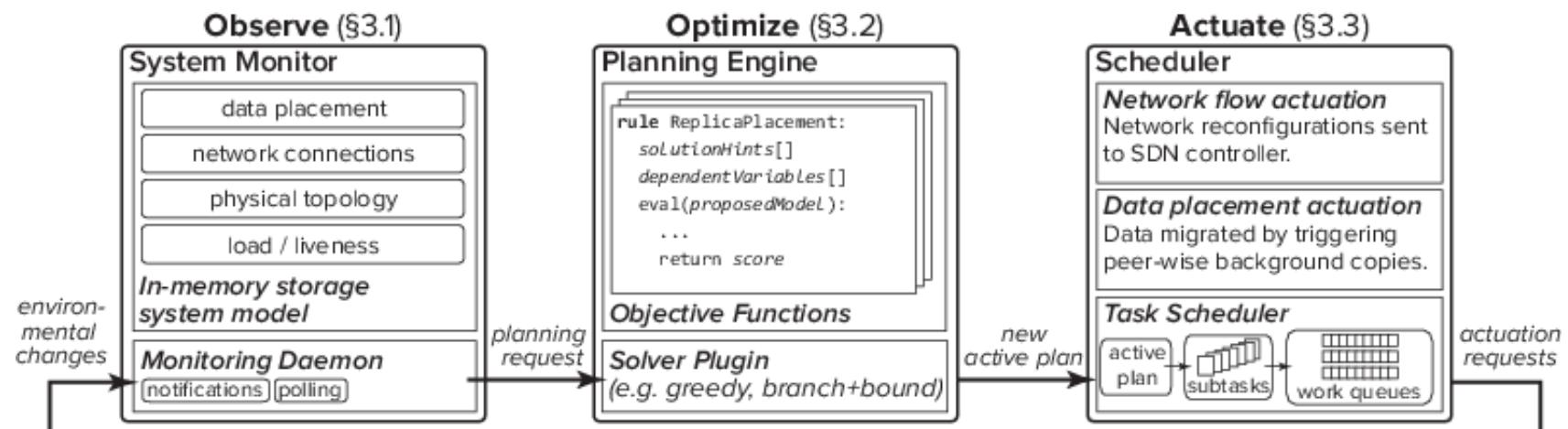
*Centralized three-stage pipeline continuously optimizes placement*
