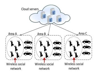
Figure 1: The architecture of the VShare carpooling system.
