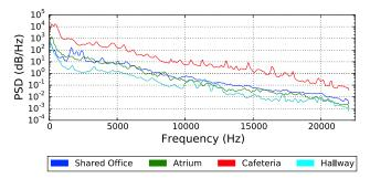
Fig. 5. Indoor Ambient Noise
