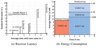
Fig. 11. Energy Consumption and Receiver Latency for Advertising.
