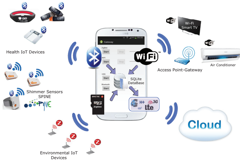
Fig. 3. Communication scenario for testing the smartphone-centric application.
