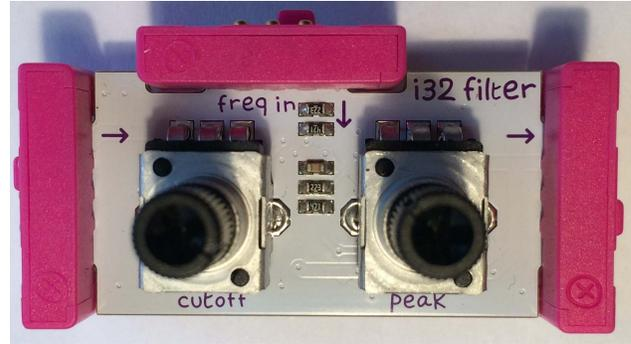
Fig. 4. A single littleBits filter module (larger than actual size).
