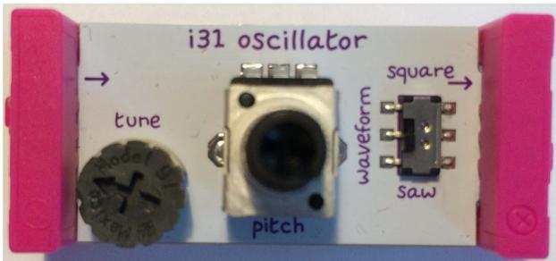
Fig. 3. A single littleBits oscillator module (larger than actual size).
