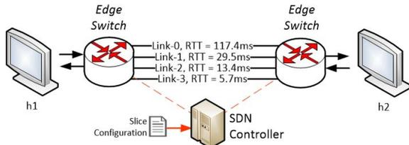
Fig. 8: Simulation setup to evaluate dynamic network slicing.
