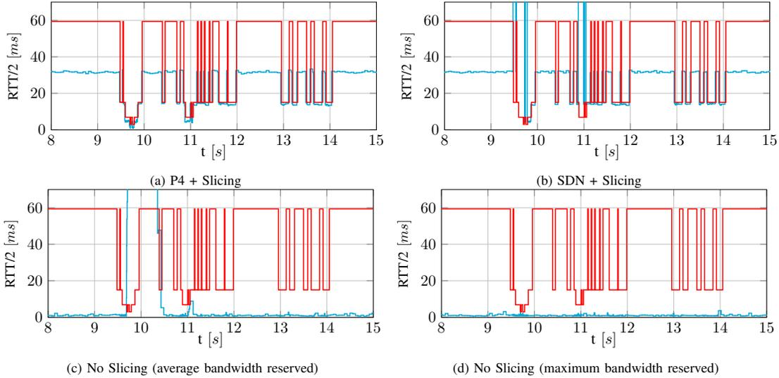
Fig. 10: Influence of external traffic: Observed one-way delay ( $RTT/2$ ) for 7 seconds of the TCPS flow when 4 slices are used for the USNET topology shown in Figure 9. Blue line represents the  $RTT/2$  measured between two TCPS edges, while the red line represents the  $RTT/2$  constraint of the current used slice determined based on the current application dynamics.
