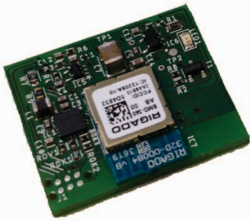
Figure 3: The FLYNC prototype based on the nRF52840. The solar panels on the backside charge a small capacitor that powers the circuit and the MCU.
