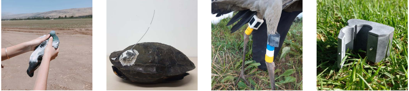
Figure 10: A tagged pigeon, terrapin, and crane. The antenna in the pigeon’s tag is a monopole; in the terrapin’s tag, a more effective dipole. The crane carries a data-logging tag with a remote release mechanism (photo taken by Petri Suorsa), shown in the released state in the rightmost picture. The VH tag and the data logger are inside the 3D-printed enclosure. The tag on the other leg of the crane is a separate GNSS tracker.
