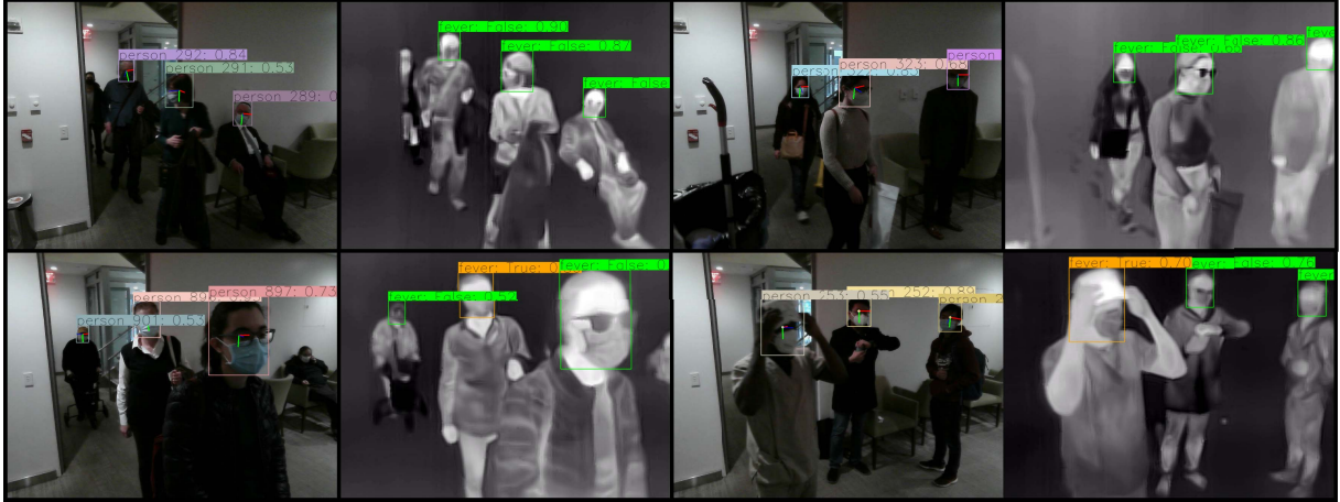
Figure 10: Real-time images available to hospital staff displaying detected people and fever screening estimates.
