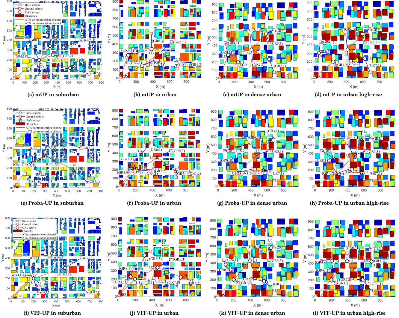
Figure 8: The placements of 5 UAVs optimized by the proposed mUP method (shown by circle lines), Proba-UP method (shown by pentagram lines), and VFF-UP method (shown by diamond lines) separately in four different types of urban environments in top viewpoint. The network composed of 5 UAVs is initialized as a star network, where each UAV connects to the BS via a direct link. There are 8 GRs and (GRm, a_m) means the m -th GR collects a_m times as much as a_0 (Mbits) data. The value of a_0 depends on specific tasks.
