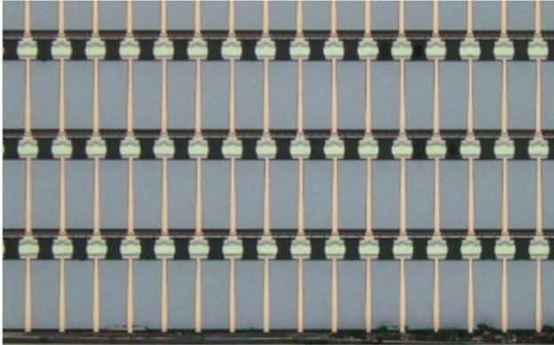
Fig. 1. Solder-based interconnection for HBM products with  $\sim 20\mu\text{m}$  pitch.
