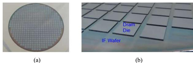
Fig. 20. Finished chip-to-wafer hybrid bonding for a fine-pitch HBM device with pics of a) full wafer and b) local image.
