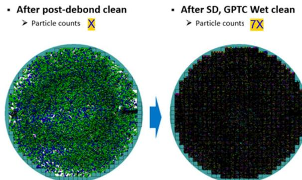
Fig. 5. Wafer particle counts increased by  $7\times$  with laser stealth dicing.
