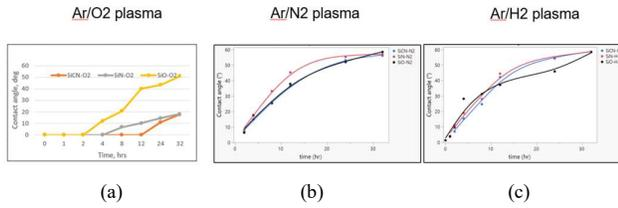
Fig. 11. Dielectric film contact angle variations with staging time after a) Ar/O<sub>2</sub>, b) Ar/N<sub>2</sub>, and c) Ar/H<sub>2</sub> plasma activation.
