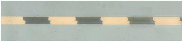
Fig. 2. Direct copper-to-copper connections for HBM.
