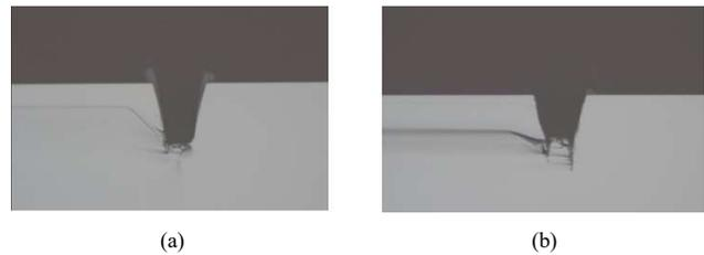
Fig. 9. Innovative cleaning to remove the laser grooving induced edge burrs and Si dust: a) before and b) post cleaning.
