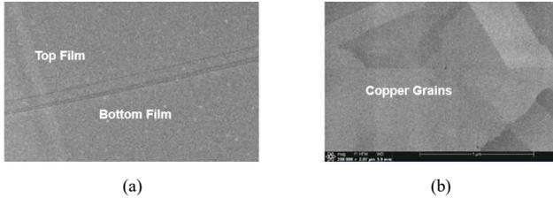
Fig. 22. Magnified images of the bonding interface between a) top and bottom dielectric films and b) Cu-Cu joints.
