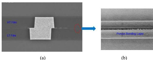
Fig. 16. Issues of low-temperature annealing with a) Cu creeping and b) porous layer between the bonding interface.
