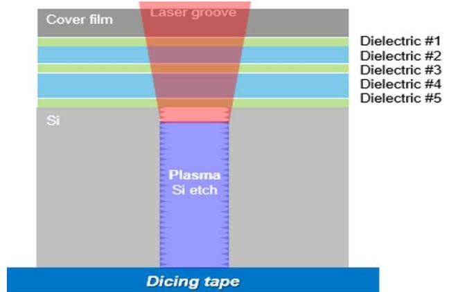
Fig. 8. Wafer dicing by laser grooving and plasma etching.
