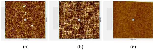
Fig. 12. Surface roughness of a) SiCN, b) SiN, and c) SiO films after Ar/O<sub>2</sub> plasma.
