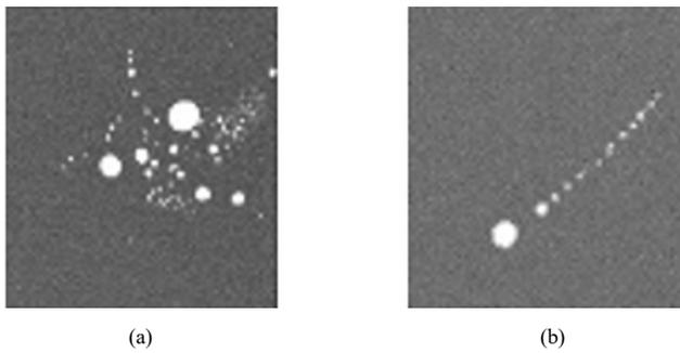
Fig. 7. Signatures of particle induced voids: a) clusters and b) comet tails.
