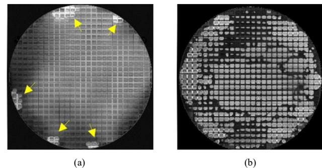
Fig. 15. a) Voids and b) delamination observed in conventional WSS with two different types of organic glues.
