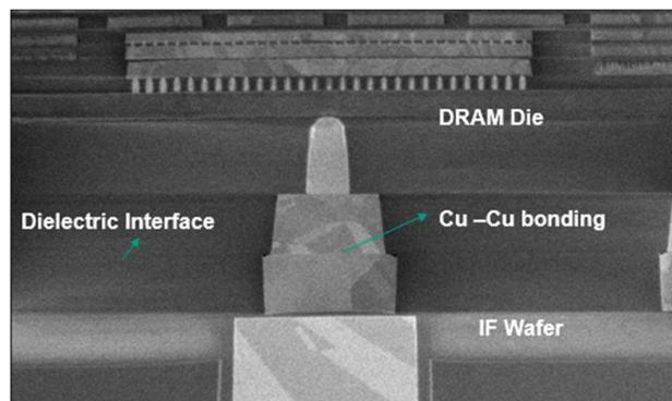
Fig. 21. X-section of copper hybrid bonding between a DRAM die and IF wafer.
