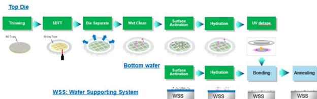
Fig. 4. HBM chip-to-wafer copper hybrid bonding process flow.
