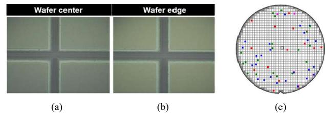
Fig. 10. Post wafer dicing images at saw streets at a) wafer center and b) wafer edge. c) Overall particle counts.
