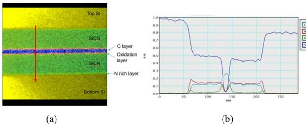
Fig. 13. a) TEM and b) EDS analysis across bonding interface of SiCN-SiCN films after Ar/O<sub>2</sub> plasma.
