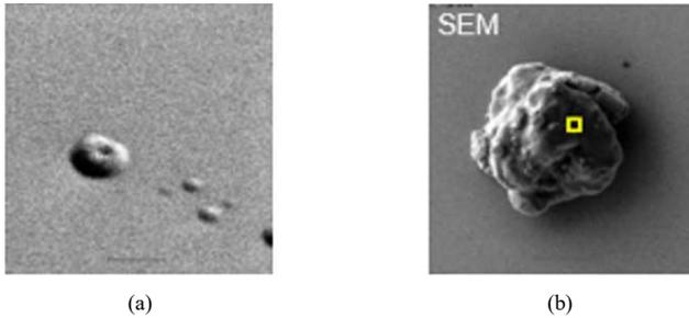
Fig. 6. Classifications of dicing particulates: a) inorganics and b) organics.
