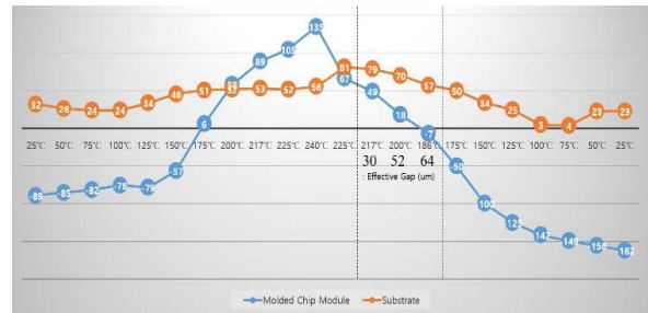
Fig 8. The results of the moiré warpage of the molded chip module and substrate warpage.
