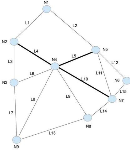
Fig. 12: Sample network with 9 nodes, where nodes (e.g.,  $N1, N2$ ) represent road intersections, and lines (e.g.,  $L1, L2$ ) represent road links. Bold lines indicate that 3 links are selected to place dynamic wireless charging pads.
