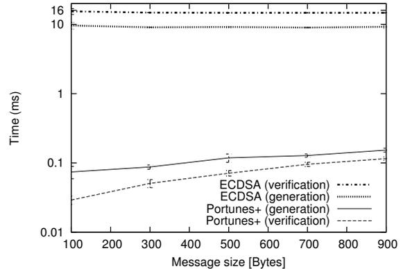
Fig. 14: Generation and verification time of authentication message using Portunes+ and ECDSA vs. message size. Error bars indicate 95% confidence intervals. The evaluation is done on Raspberry Pi 2 Model B.
