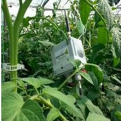
Figure 3. Wireless sensor node in a greenhouse.
