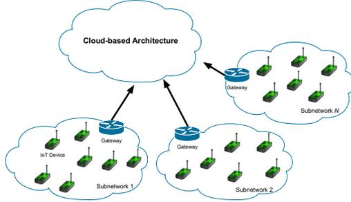
Figure 1: A cloud-based IoT network model.
