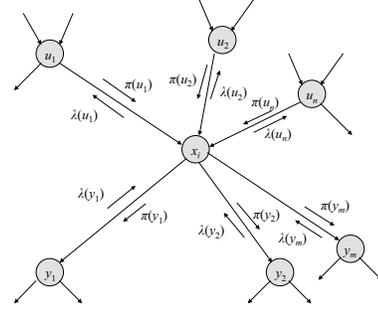
Figure 3: Architecture of the IoT Bayesian network as a graph, for the computation of the BP algorithm.
