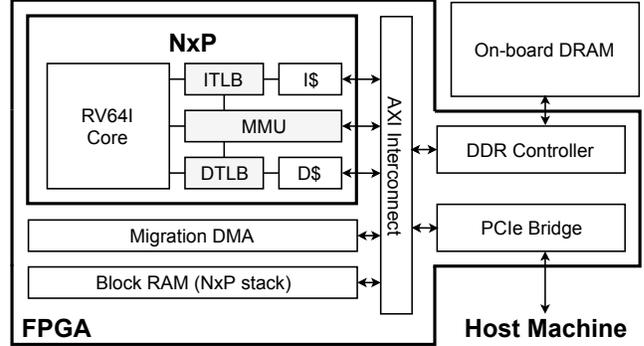
Fig. 4. FPGA-based evaluation platform for Flick.
