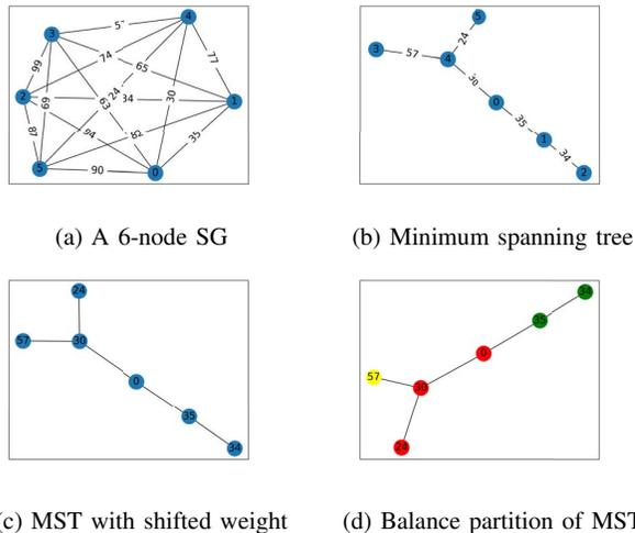
Fig. 9: The procedure from  $SG$  to partitioned  $MST$ : extract  $MST$  (b) from  $SG$  (a); shift the weight on edges to nodes (c); partition the graph into several balanced groups of similar sum of node weight, denoted by a distinct color (d).
