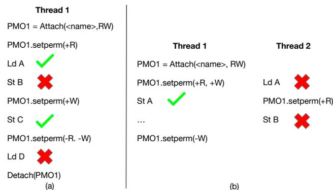
Fig. 2. Example of: (a) Intra-thread (temporal) protection (b) Inter-thread (spatial) protection.
