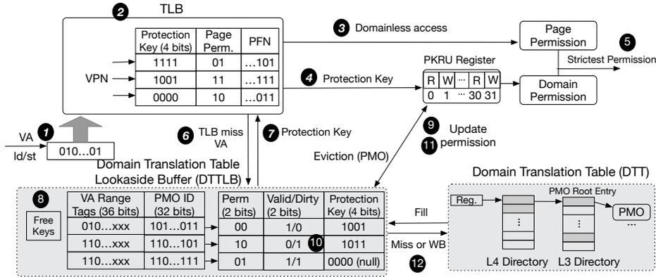
Fig. 4. Diagram of the MPK virtualization scheme.
