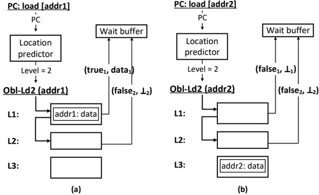
Fig. 3: Example Obl-Ld operation given two different addresses  $addr1$  (present in L1) and  $addr2$  (present in L3). In both cases, resource contention and operation timing is a function of the prediction, not the address.
