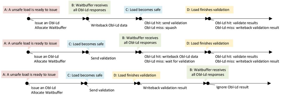
Fig. 4: Obl-Ld operation flow with the three possible event sequences (top:  $A < B < C < D$ ; middle:  $A < C < B < D$ ; bottom:  $A < C < D < B$ ) and corresponding actions.
