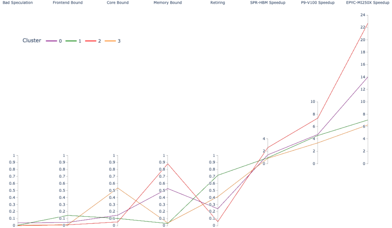
Fig. 8: Parallel coordinate plot showing average top-down metrics and speedup over SPR-DDR per cluster. The average of each of the top-down metrics per cluster is shown in the first five axes and then average speedup per cluster in the last three axes. Cluster 2 (red line), made up of primarily memory bound kernels, exhibits the highest speedup on all architectures.
