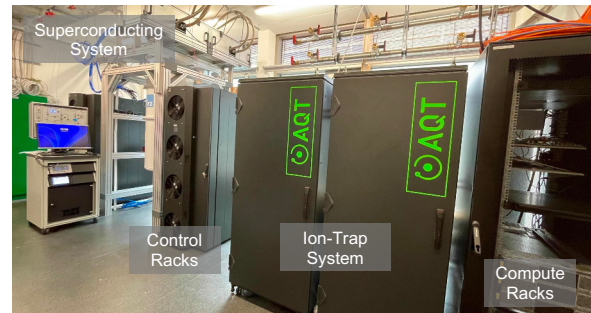
Fig. 1: A view into the Quantum Integration Centre (QIC) at LRZ/Munich showing a superconducting system (left), an ion-trap system (middle) and HPC racks covering the classic compute. The result is a strongly disaggregated infrastructure combining classical HPC clusters with large-scale accelerator appliances, which nevertheless need to operate as a seamless, single system.
