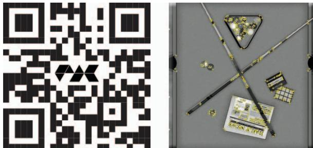
Figure 2: A customized QR code (left) can both encode information or be used as an anchor for marker-based tracking. A *Vuforia* image-based marker (right) utilizes a number of unique, asymmetrical edges.
